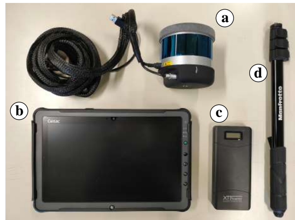
Figure 1. Main components of the HERON Lite handheld system. (a) Sensor head (Velodyne Puck LITE laser scanner + XSens MTI IMU), (b) control unit, (c) battery, (d) telescopic pole.
