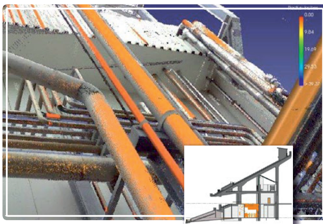
EdgeWise MEP pulled 90-95% of pipes accurately - lengths, elbow angles, and sags in long pipe runs included.
