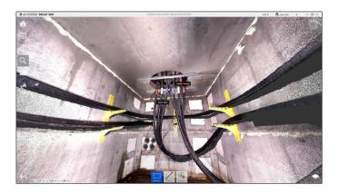
The resulting point cloud models have improved the efficiency and accuracy of the design process for ML&P. These models are used to take internal measurements, verify conduit and conductor configurations, verify equipment statuses and locations, and as an accurate 3D reference in AutoCAD, allowing engineers to design to accurate real world conditions.
